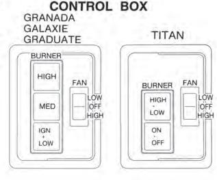
The Titan high burner control button may be in either position for ignition.
