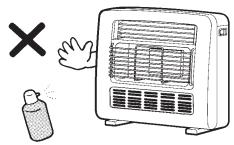
Use of aerosols, paint, polishes, etc., while this heater is in use may cause unpleasant smells. Most aerosols contain butane gas, and can be a fire hazard if used near this heater when it is in use.
