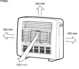
Do not allow curtains or other flammable materials to come into contact with the heater.
